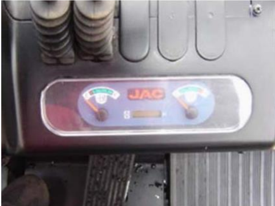
5. The instrument panel of the diesel powered lift truck is installed at right hand side. The simple design makes it easier for the operator to read the parameters.
